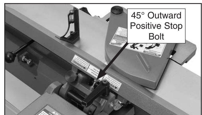
Figure 76. Adjusting fence 45° outward.
